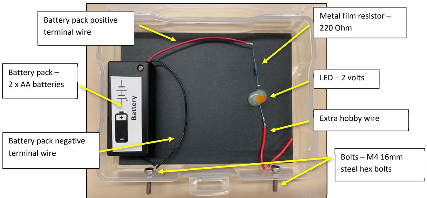
To focus attention on the design of creative switches with a specific purpose and user in mind, we built robust and safe circuit boxes. You could include creating the circuit as part of the activity.
